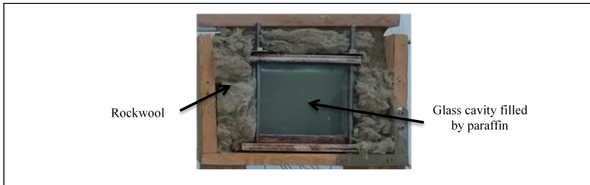
Figure 1. Thermal cavity isolated by Rockwool.
